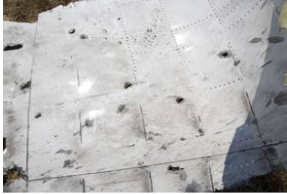
Machine gun fire on outer fuselage
